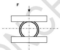
Figure 1 – test set-up for compression
