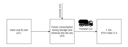
Figure 1: Simplified process flow chart of the production of EFA-Füller<sup>®</sup> D 4
