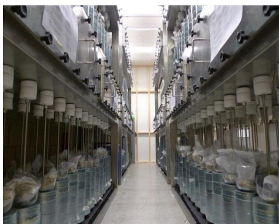
Figure 6 – Full-scale set-up (30 mbar(g)) used to determine the effects of sustainable gases on polymeric materials
