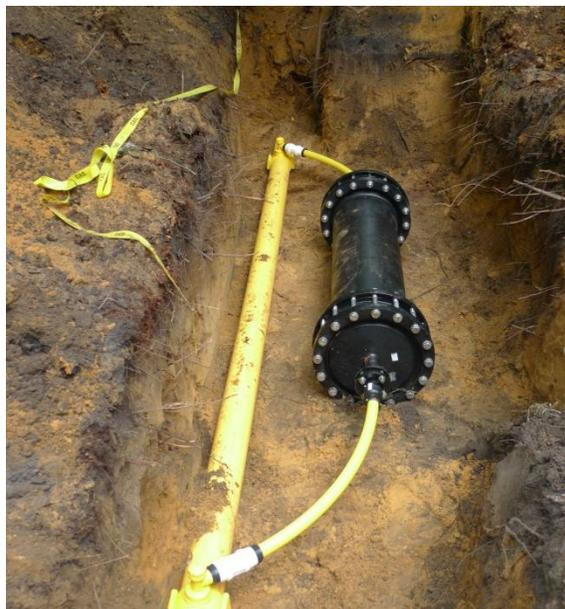
Figure 10 – Test rig for G-gas
