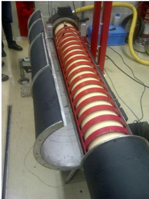
*Figure 3. Test rig for hydrostatic S4 tests. Inside the PVC segment a water/glycol mixture flows to cool to 3 °C. Cooled air of 3 °C flows through the insulated steel jacket pipe (shown in open position).*
