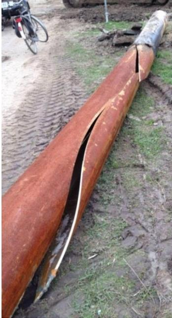
Figure 1. PVC water pipe with a long brittle crack due to RCP.
