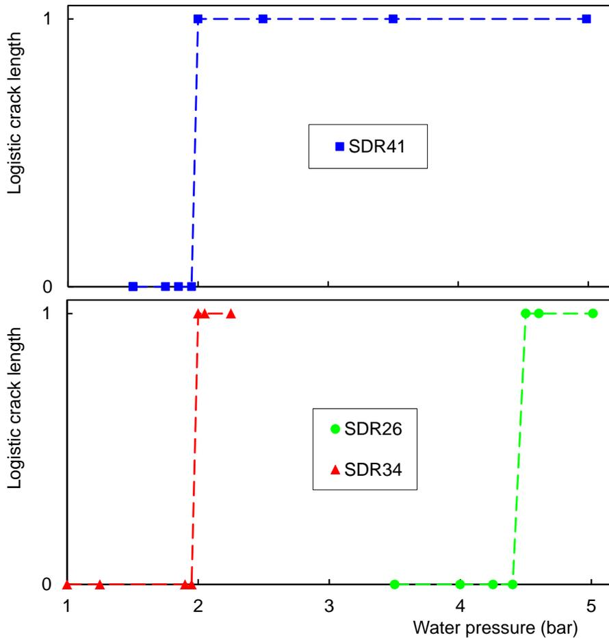
Figure 11. Description of the logistic crack length (L) of SDR41 segments with the statistical model. The same model with the same coefficients was used for Figure 12.
