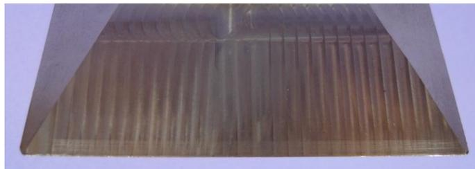
*Figure 4. Steel knife 120 mm wide which falls on top of the segment to initiate the crack. The knife was weighted to 36 kg. The width of the knife was aligned with the longitudinal direction of the pipe.*
