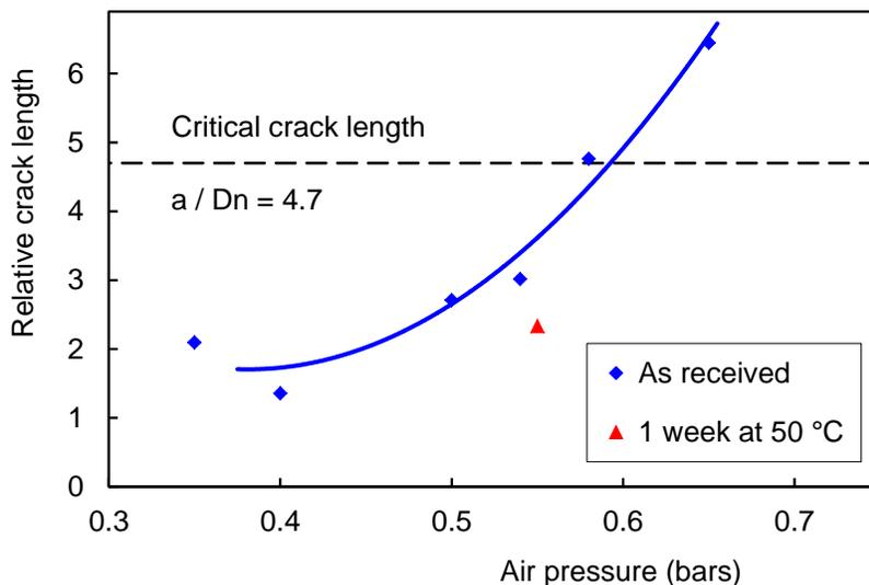
Figure 14. Relative crack length in the pneumatic S4 test as a function of the air pressure<sup>[15]</sup>, measured on 315 mm SDR41 pipe segments at 0 °C.  $P_C$  in air is 0.53 bars at these pipe dimensions. The red point is from a segment in which the residual stress had been released by oven ageing during 1 week at 50 °C. There are five cases of arrest.
