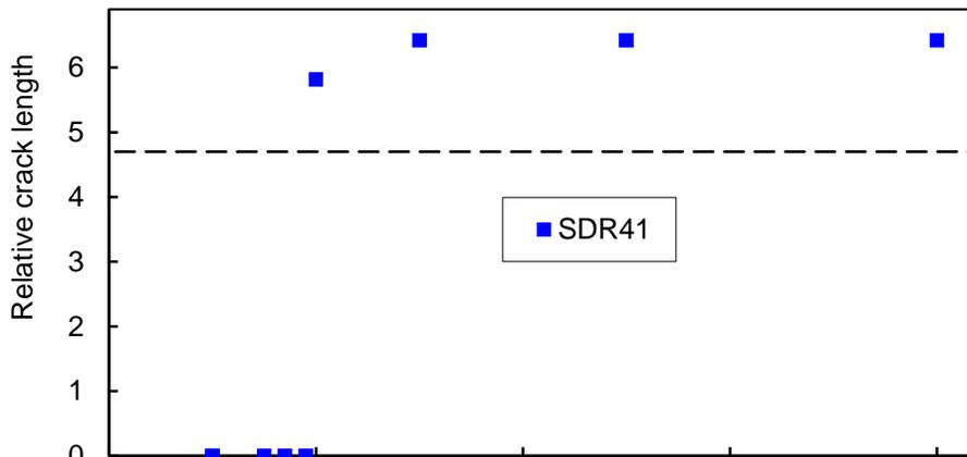
Figure 7. Relative crack length in the hydrostatic S4 test as a function of the water pressure in SDR41 pipes.  $P_C = 1,95$  bar.
