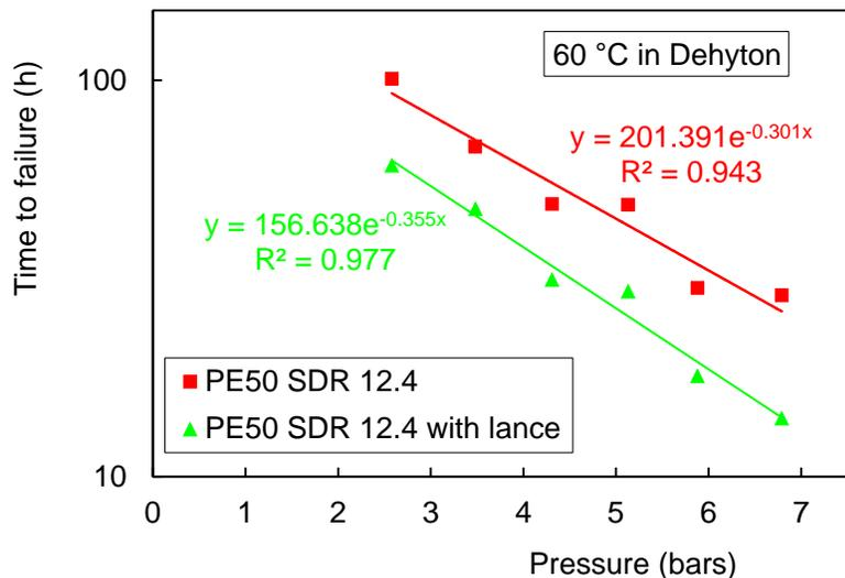
Figure 10. A reduction of the time to failure by about 40% when the turbulence of the detergent solution inside the tested pipe segment is increased. Measured on SDR12.4 PE50 pipe segments at 60 °C in 2% Dehyton PL in water.
