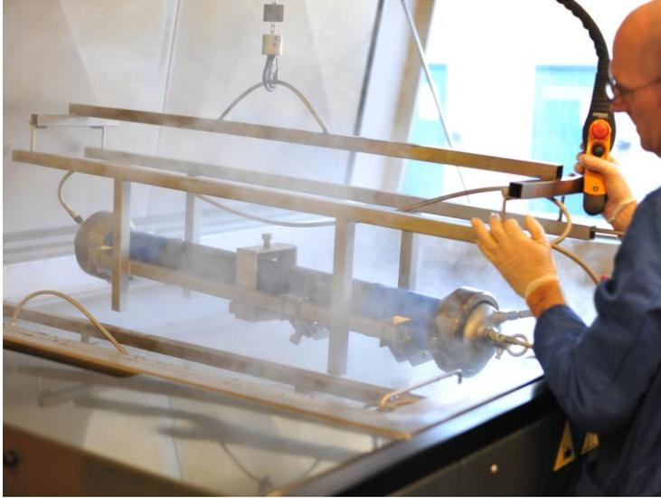
Figure 4. Execution of the PLT. The PE pipe segment is hydrostatically tested with a 2% detergent solution pumped through the inside and an additional point load on the external surface in the middle.
