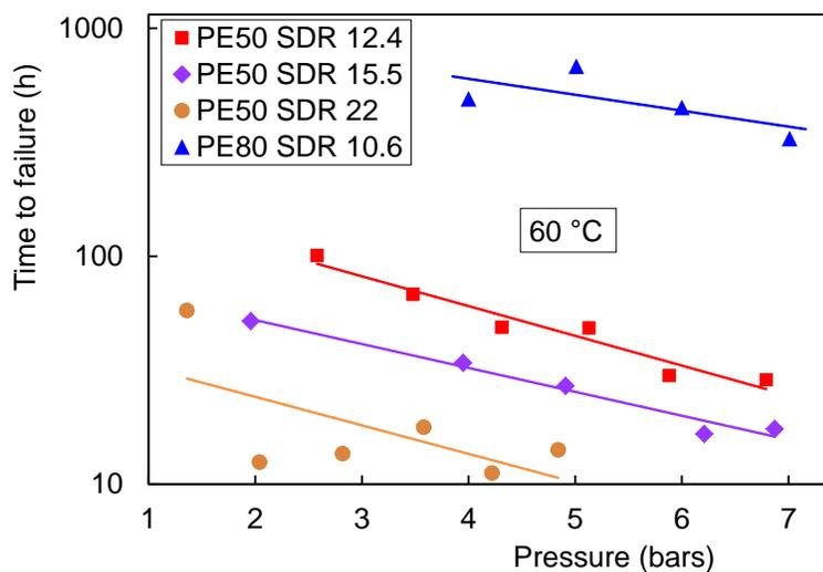
Figure 8. Addition of the results from the PLT on PE80 HDPE pipes at 60 °C to Figure 7.
