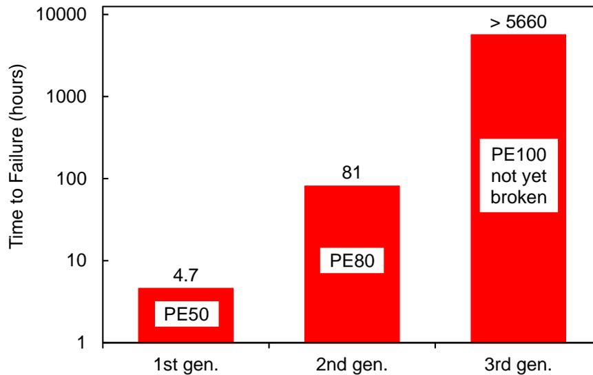
Figure 9. Failure times in the PLTs on three generations of HDPE pipes at 4.0 MPa hoop stress at 8 mm indentation and at 80 °C. The PE50 pipe is SDR12.4, the PE80 HDPE pipe is SDR11. The SDR11 PE100 pipe has not yet failed.
