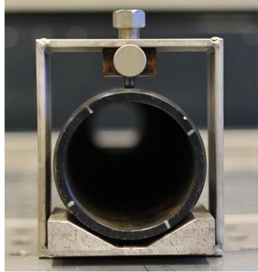
Figure 5. The point loading tool at the top (diameter 10 mm with round top) and the support at the bottom. A 110 mm PE pipe is placed in between.
