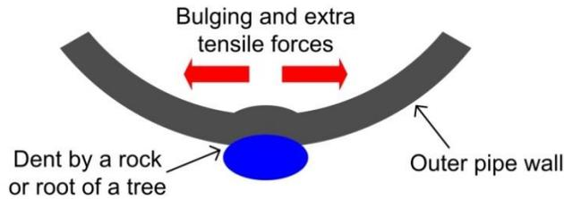
Figure 3. A point load acting externally on a PE pipe leads to additional tensile stresses on the inside of the pipe (schematic). These additional tensile stresses lead to premature failure, with respect to the situation without point loads.
