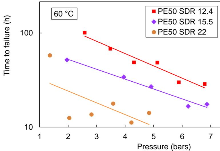
Figure 7. Failure times for 110 mm PE50 pipes with three SDR values in the PLT at 60 °C plotted as a function of the internal pressure. When the SDR increases (the wall thickness decreases), the time to failure decreases.
