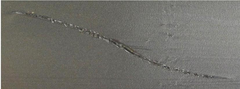
Figure 2. Brittle failure on the inner surface of an excavated PE50 gas pipe due to a point load. The failure occurred in practice. The crack on the inside of the pipe bore is 75 mm long but the crack on the external surface is only 1 – 2 mm (not shown). The axial pipe direction is horizontal.
