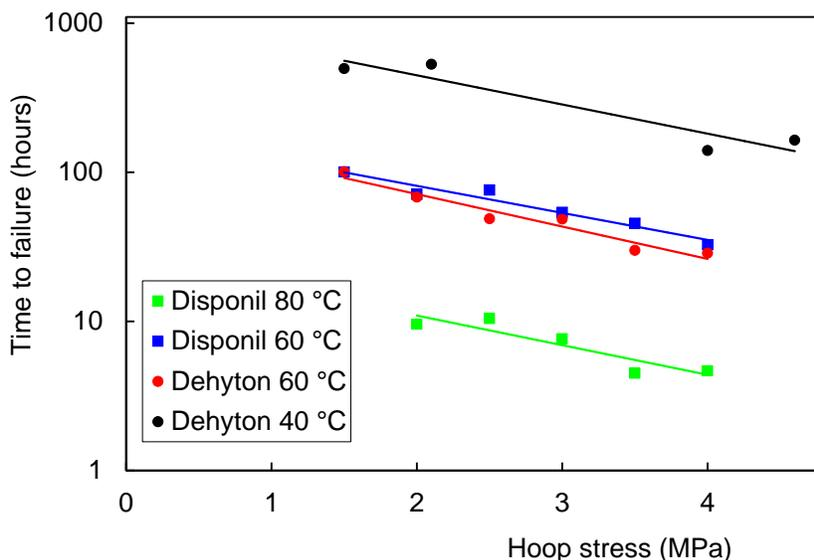
Figure 6. Influence of the hoop stress (calculated from the internal pressure) and the testing temperature using two very similar detergents, at 8 mm indentation of the point load.
