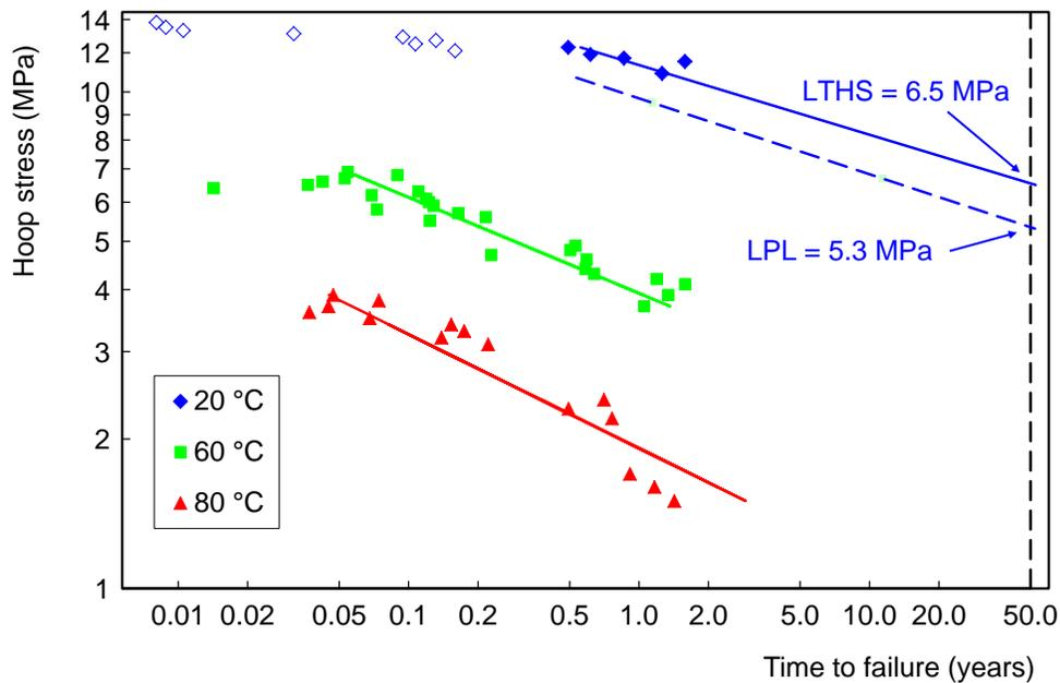
Figure 1. Internal Water Pressure tests evaluated according to ISO 9080 on excavated German PE50 gas pipes, after 32 years of use. Reproduced from [1]. Open symbols: ductile failures, closed symbols: brittle failures. The Lower Probability Limit (LPL) proves the MRS class was still above 5 MPa.
