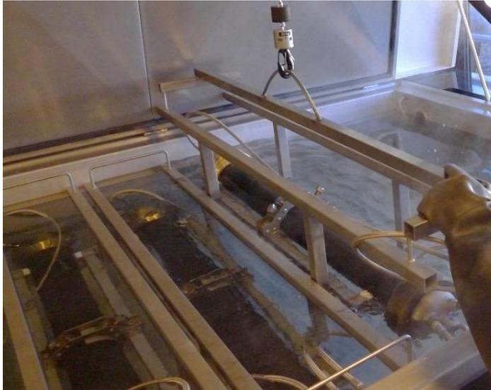
Figure 8. Execution of the PLT. The PE pipe sample is hydrostatically tested with detergent inside and a point load on the external surface.
