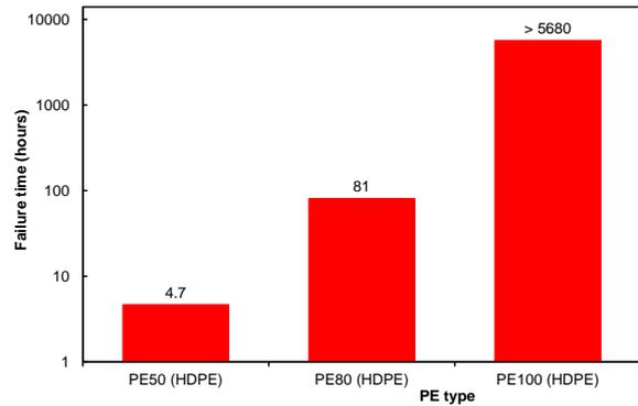
Figure 11. Times to failure in point load test for various PE grades. The test was performed at 80 °C in Disponil.
