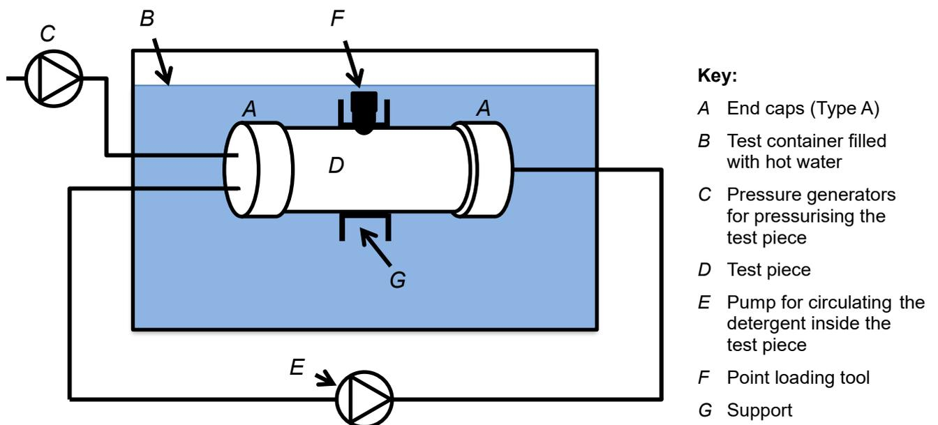
Figure 7. Test setup for the application of the external point load and the hydrostatic internal pressure.
