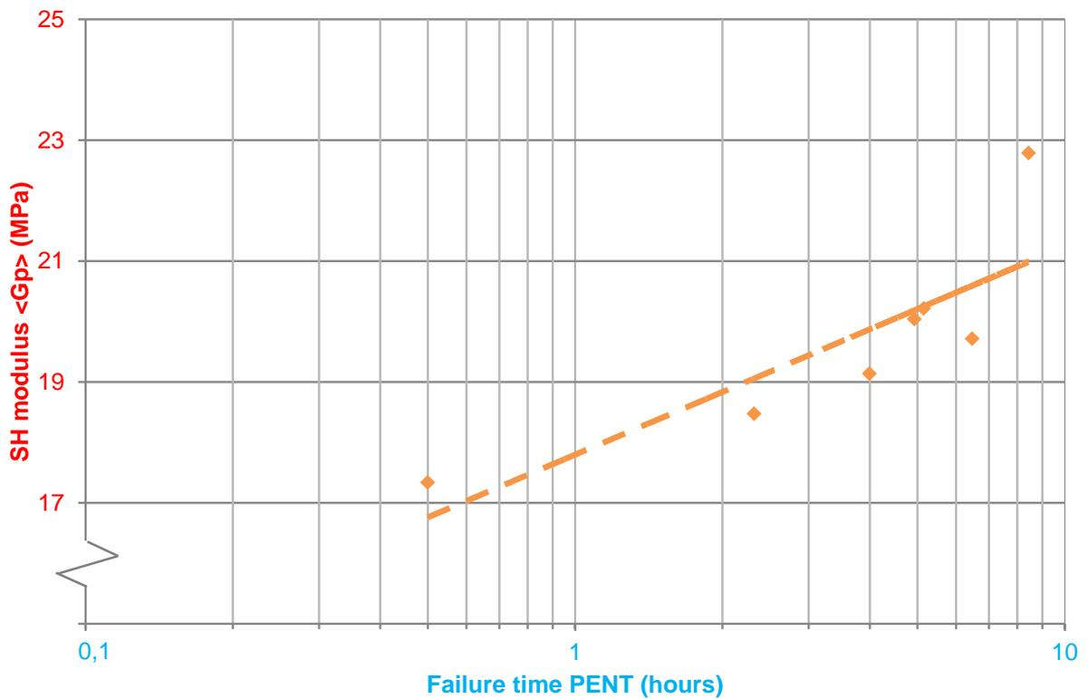
Figure 6. Correlation between the SH test (<Gp>, vertical axis, red) and the PENT (horizontal axis logarithmic, light blue).
