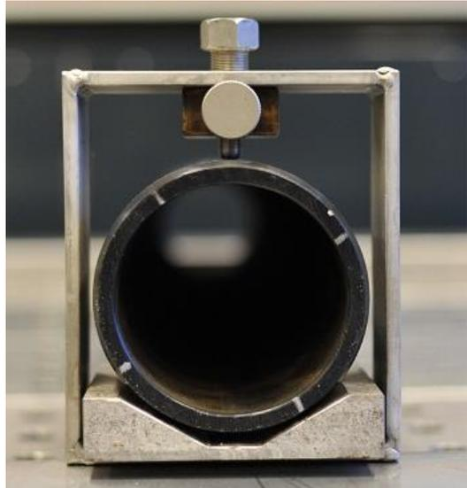
Figure 9. The point loading tool at the top and the support at the bottom. A Ø110 mm PE pipe is placed in between.
