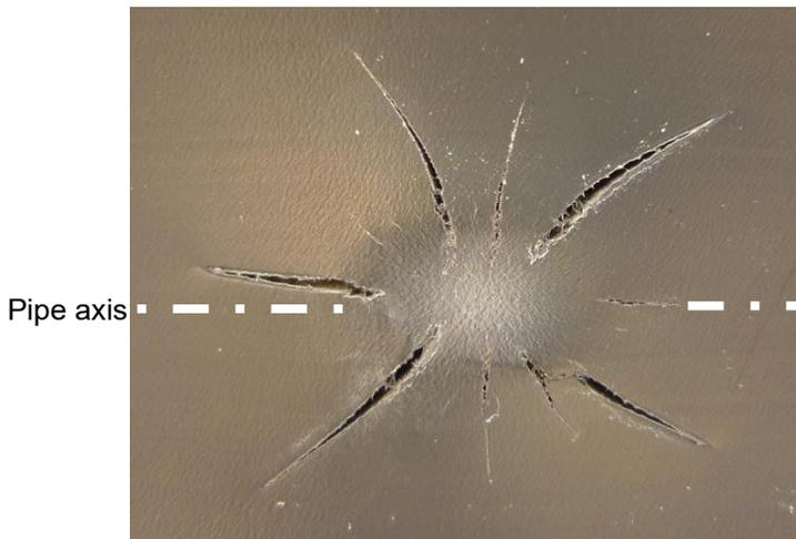
Figure 13. The inner wall of a second generation PE pipe after the PLT at 80 °C and 8 mm indentation in Dehyton shows multiple cracking. The cracks start just next to the centre of the indentation where no yielding occurs.
