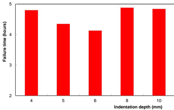
Figure 10. Time to failure for various indentation depths of the point load for first generation PE grades (PE 50) at 80 °C in Disponil. The average failure time is 4.7 hours.
