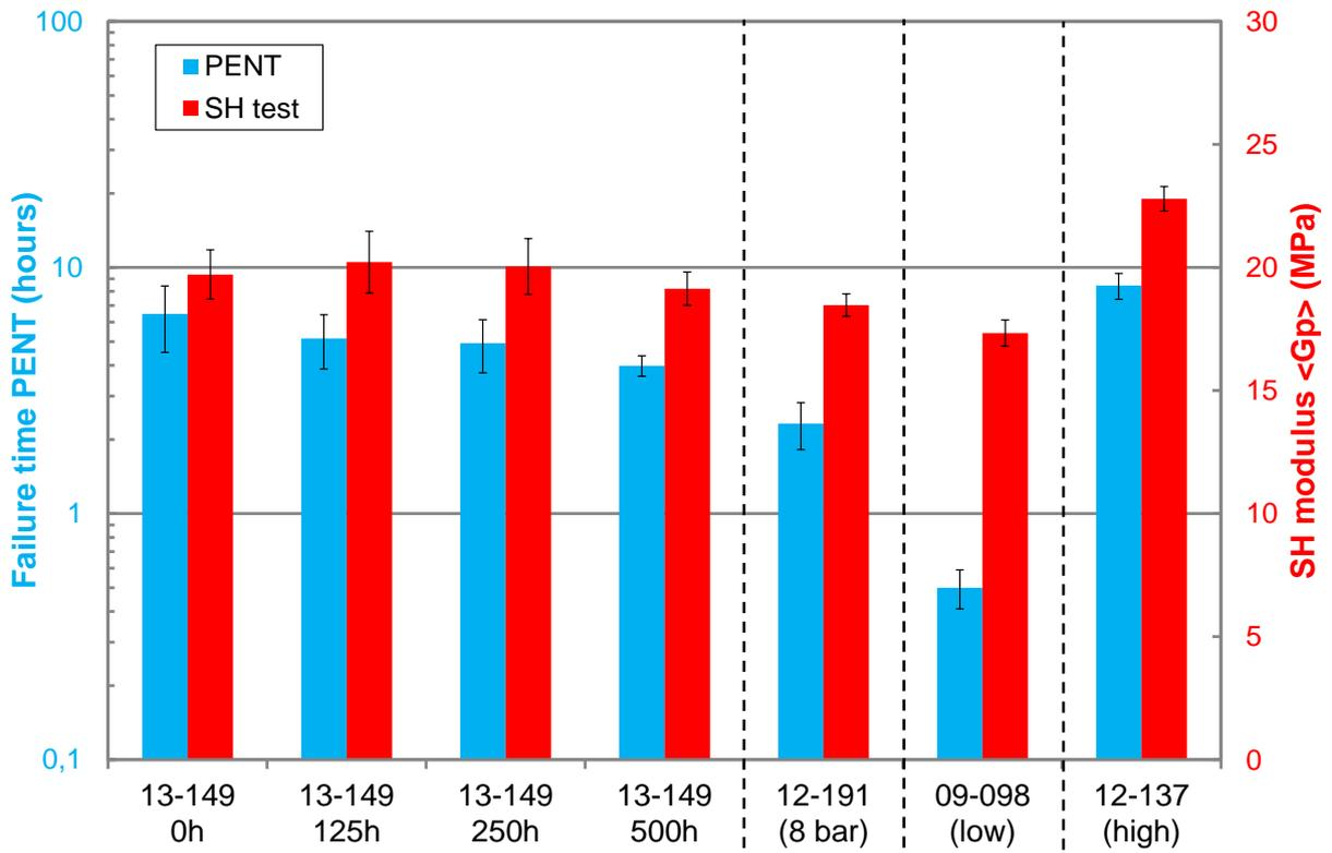
Figure 5. The failure time of the PENT (left axis on logarithmic scale, light blue) and the strain hardening modulus of the SH test (<Gp>, right axis, red).
