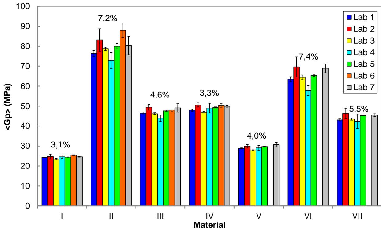
Figure 3. Results of a Round Robin test performed by seven laboratories on seven PE materials in which each laboratory prepared its own 1 mm thick samples. The coefficient of variation (the relative standard deviation) based upon all individual samples is given above the histogram of each material.
