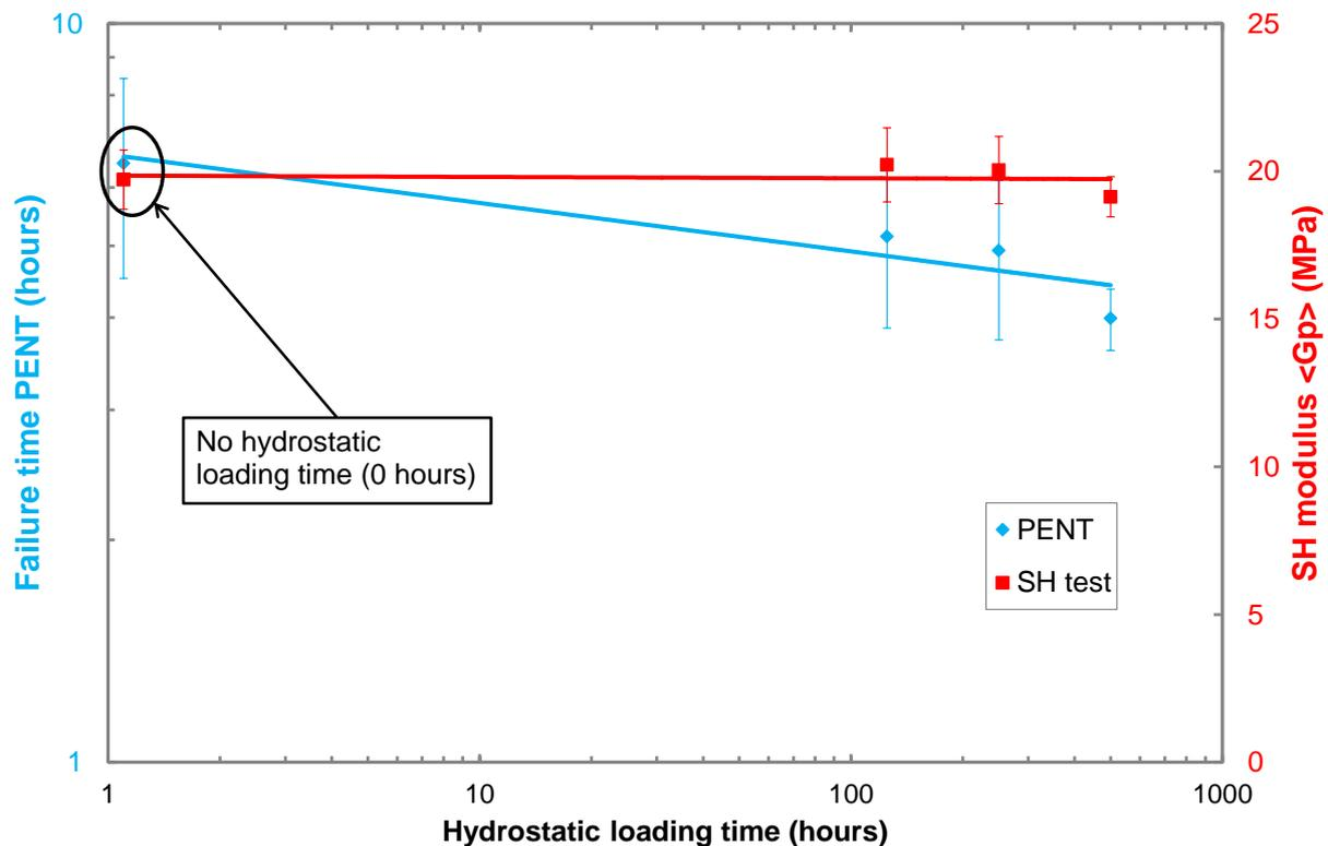
Figure 4. The failure time for the PENT (left axis on logarithmic scale, light blue) and the strain hardening modulus of the SH test ( $\langle G_p \rangle$ , right axis, red). The hydrostatic loading time is shown on the horizontal axis (logarithmic). There is no “0” on a logarithmic scale; the value without hydrostatic loading is thus placed at 1.1 hours for clarity.
