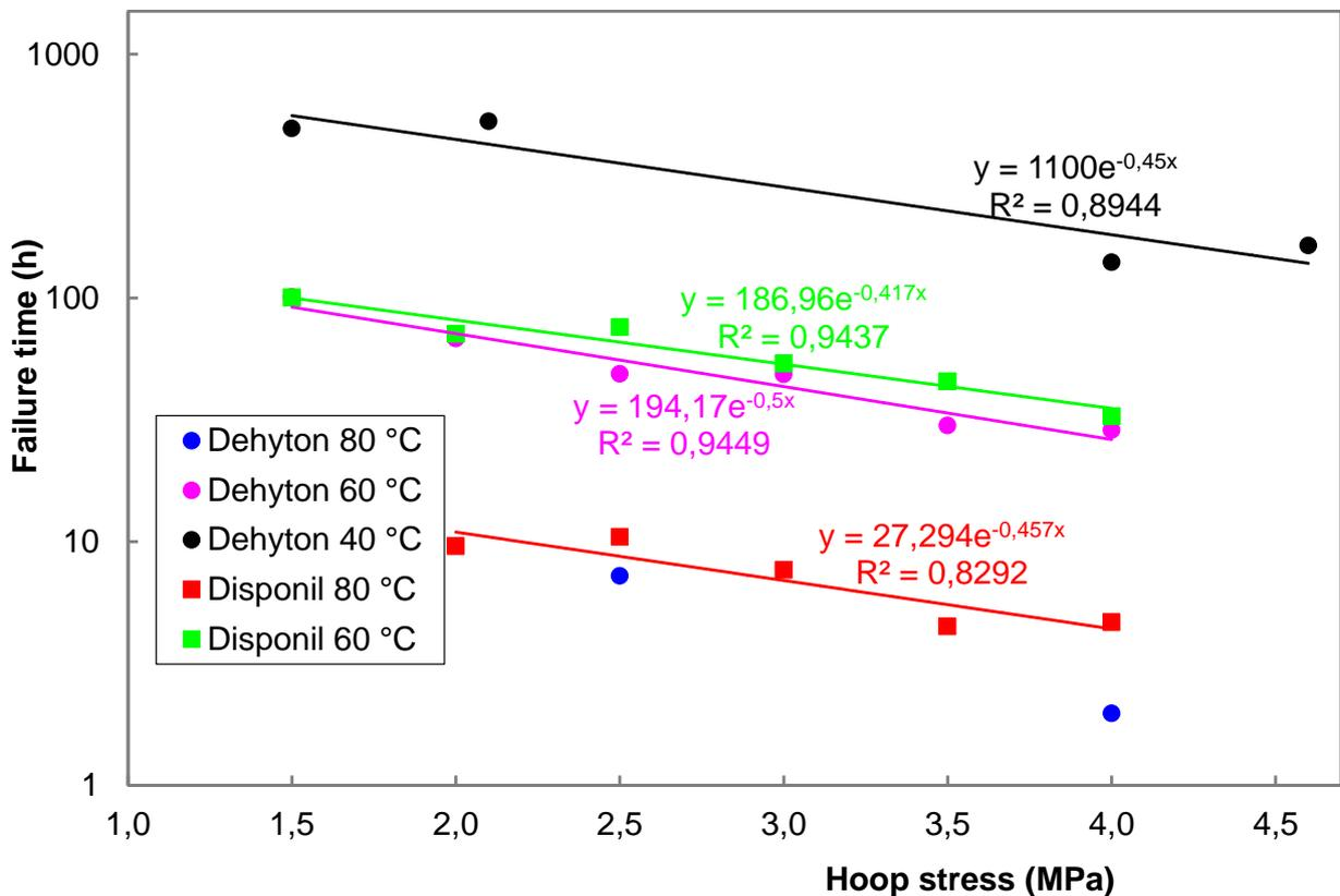
Figure 12. Comparison between the detergents Dehyton and Disponil at different hoop stresses and temperatures, using PE 50 pipes and an indentation depth of 8 mm.
