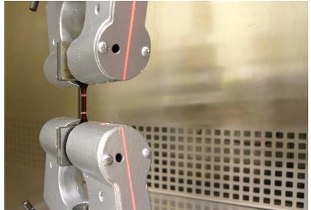
Figure 2. A SH sample ready for testing using a laser extensometer.
