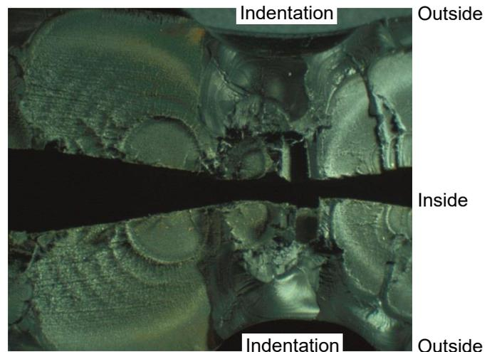
Figure 14. Brittle fracture surfaces after the PLT at 4.0 MPa and 80 °C in Dehyton. On the left the concentric ovals typical for slow crack growth are present.
