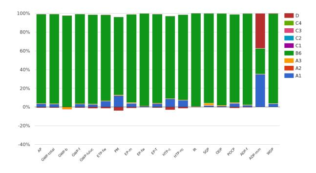
As can be seen in the graph, for all environmental impact categories, module B6 (operational energy use) has the biggest influence. This is due to the fact that this module has been calculated for the whole reference service life of the product (50,000 hours).
