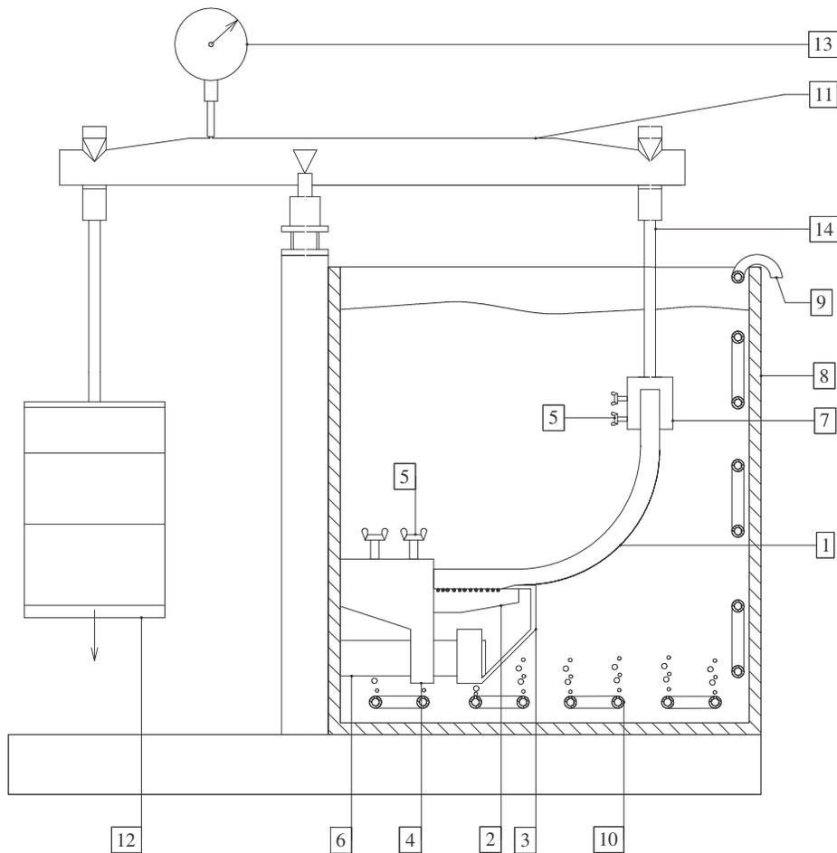
Figure 2. Principle of the Slow Peel Test.
