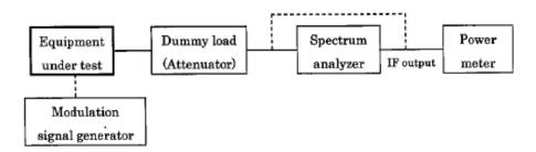
Note 1: The power meter is directly connected to the dummy load output for measuring total power in a system other than orthogonal frequency division multiplexing system and spectrum spreading system using direct sequence spreading.
