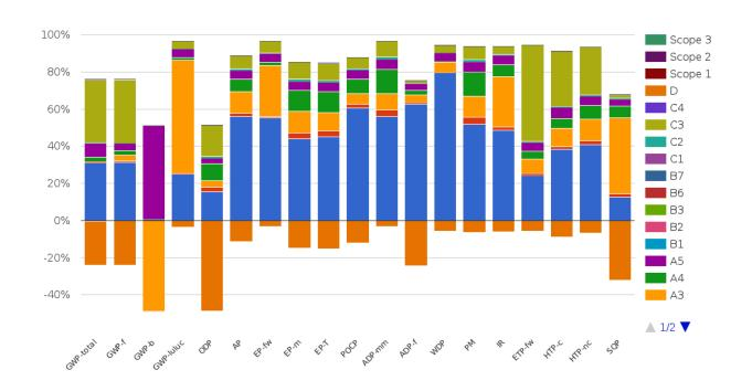
It has been analysed what the contribution is of the modules to the total GWP per functional unit. In the next table it is shown which phase(s) contribute(s) most and how much (the (high) contribution of module A1-A3 is mainly due to module A1 (raw materials)):
