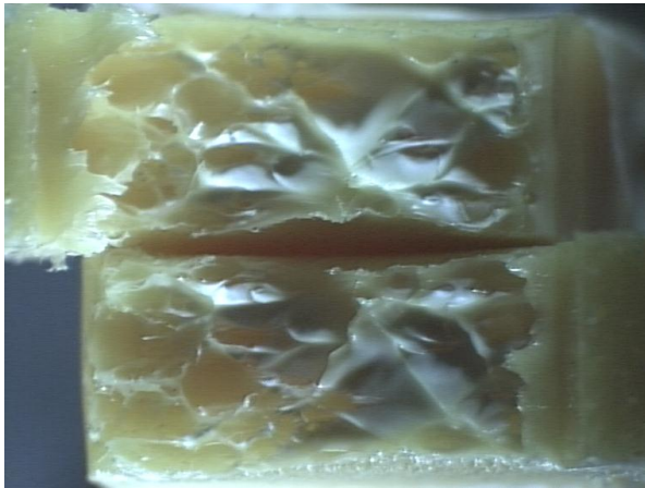
Figure 3. Broken test bar B8 from a previously water-saturated butt fused PA pipe (type A) after 153 hours of Constant Load testing at 15 MPa and 100 °C.
