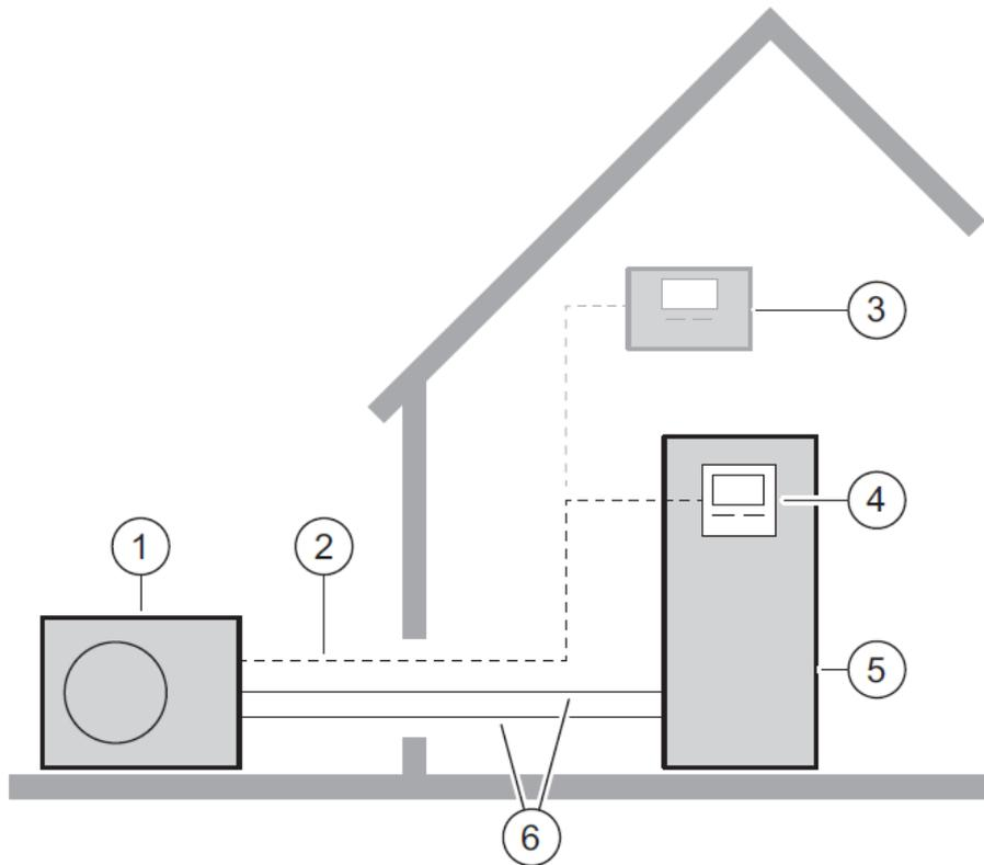
**Figure 1: Structure of a typical heat pump system with monobloc technology**
