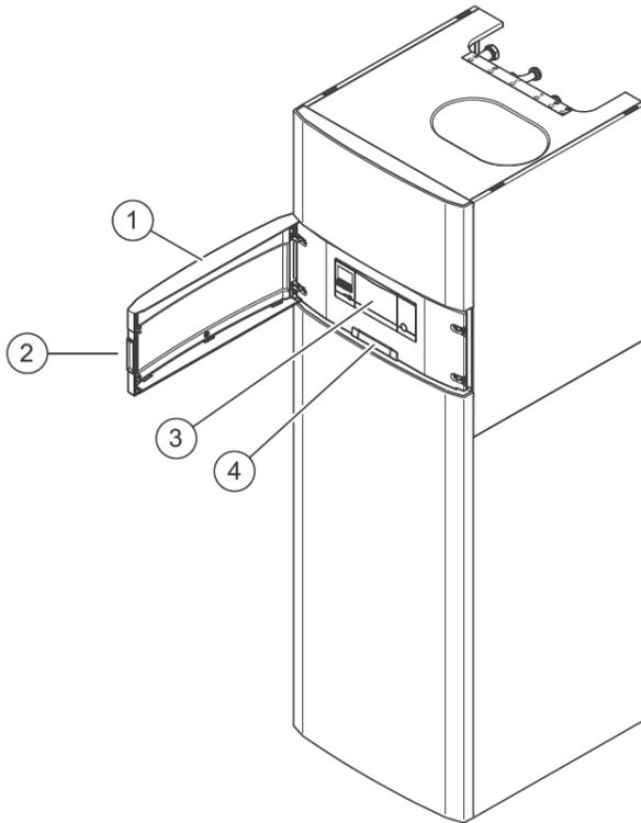
**Figure 3: Structure of the product uniTOWER plus**
