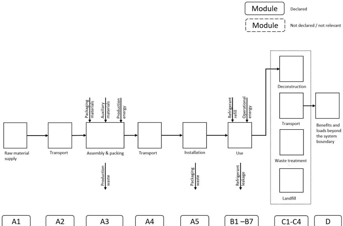
**Figure 4: Process flow chart for aroTHERM plus 7 kW & uniTOWER plus**
