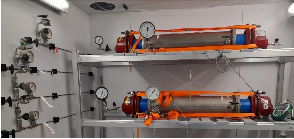
Figure 1. Sealed PVC pipe surrounded with a steel jacket pipe for the permeation measurement in a temperature-controlled room.
