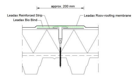
Figure 2 - Overlap connection roofing membrane
