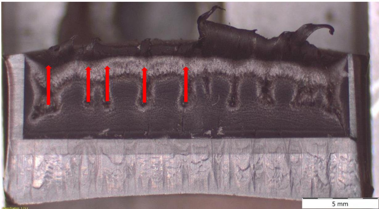
*Figure 9: PENT test fracture surface of PE 2022-229#1. Lines can be distinguished. These are indicated with red arrows and probably arose during the formation of the ductile fracture.*
