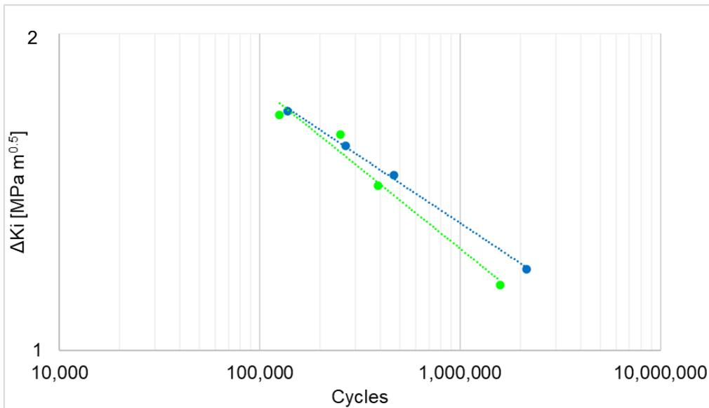
Figure 4: CPENT test failure cycles vs. stress intensity ( $\Delta Ki$ ) for a pipe material in blue and the same pipe aged for 800 hours in green.
