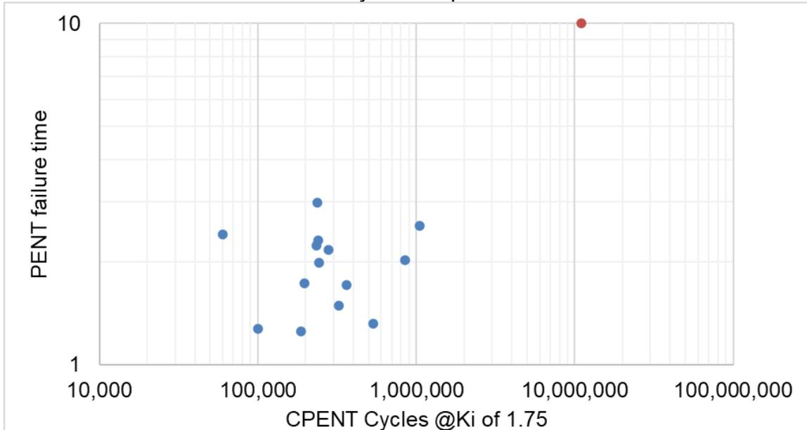
Figure 5: PENT test failure time vs. CPENT test cycles @ $K_i$  of 1.75. The red data point represents a second-generation material that did not fail during the PENT test.
