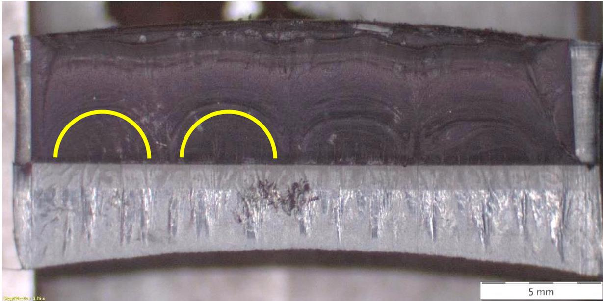
*Figure 8: CPENT test fracture surface of PE 2021-268#4. Four semicircular zones can be distinguished. These appear to be distinct initiation points. Two of the four zones are indicated with yellow semicircles.*
