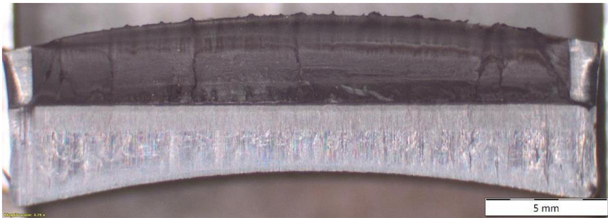
Figure 7: CPENT test fracture surface for PE 2022-311#3. The different SCG are difficult to distinguish.
