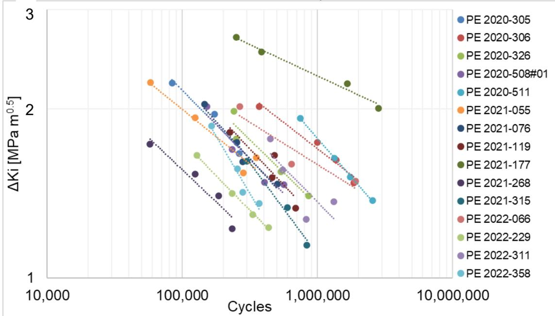
Figure 3: CPENT test failure cycles vs. stress intensity ( $\Delta Ki$ ). The dotted line shows a fit between the four tested specimens.
