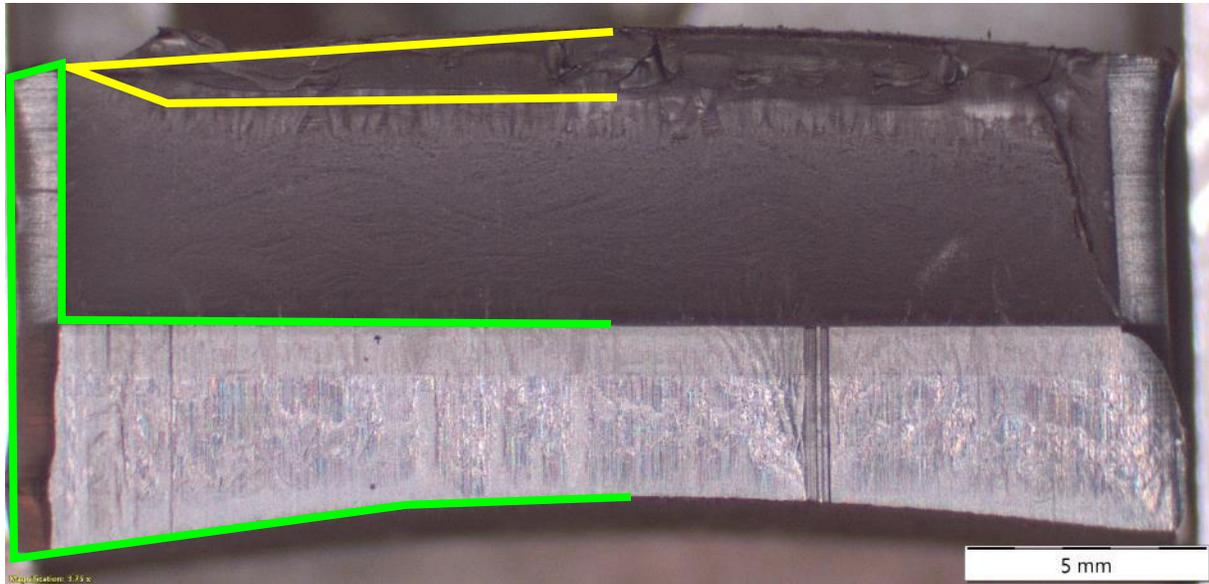
Figure 6: CPENT test fracture surface for PE 2022-229#2. The notch made with a razor blade is shown in green. The final ductile fracture is shown in yellow. The area in between is the smooth surface, which represents slow crack growth.
