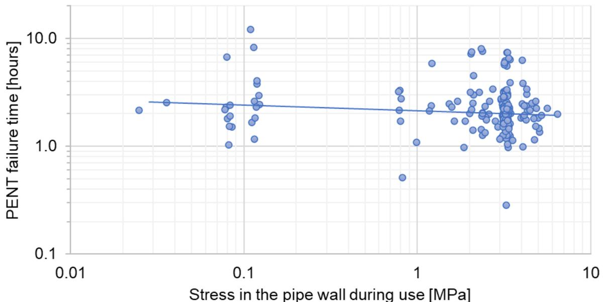
Figure 2: PENT test failure times and the stress in the pipe wall.
