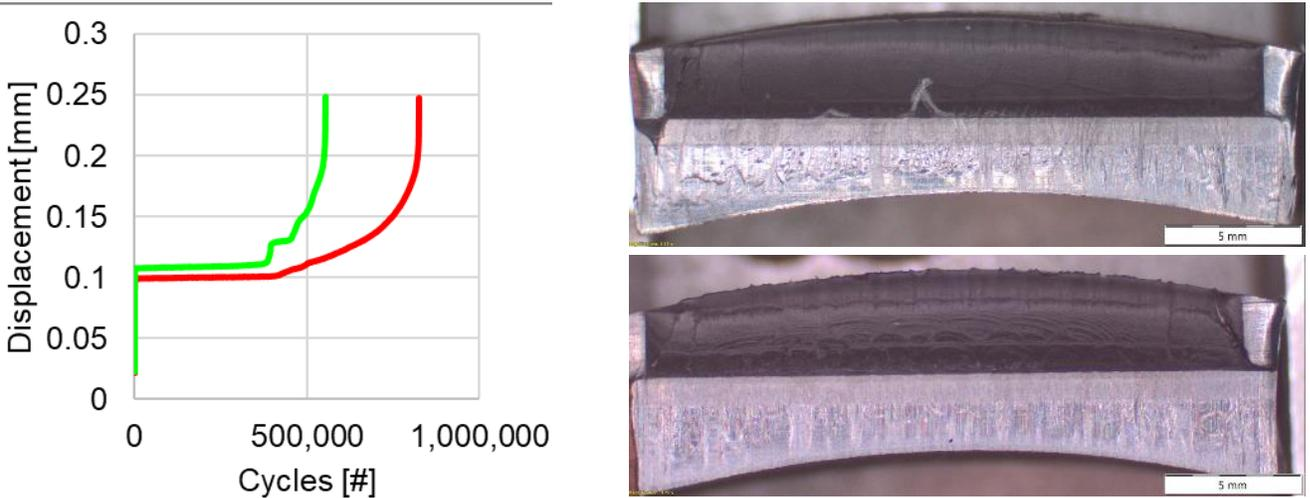
Figure 10: Left the displacement vs cycles of CPENT PE 2022-311. #1 in red and #4 in green. On the top right the fracture surface for #1 and bottom right for #4.
