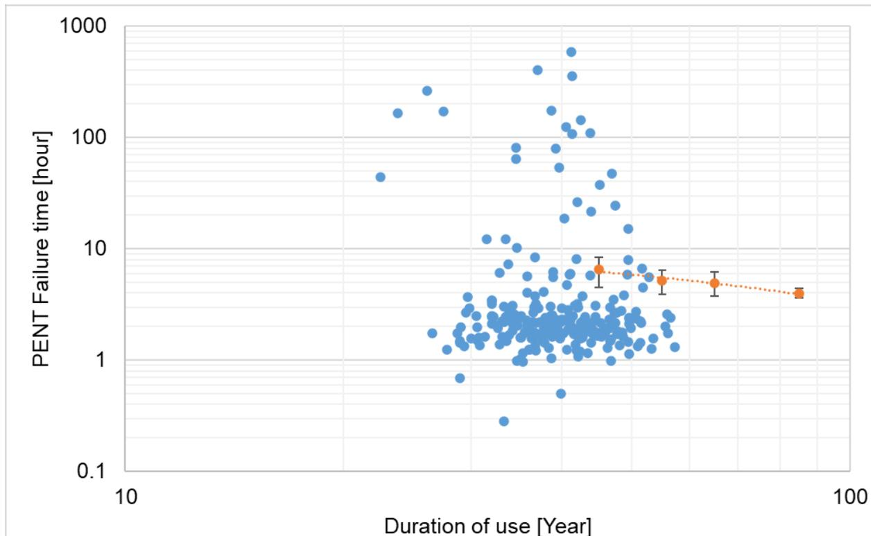
Figure 1. PENT failure times of tested pipes and PENT failure times of an artificially aged pipe.
