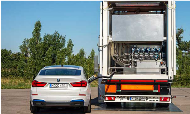
Photo: The BMW 5GT fuel cell vehicle and a mobile filling station for 350-bar cryo-compressed hydrogen gas. The 'CC' on the license plate refers to the storage method. The BMS's air inlet and water vapor outlet are highlighted in blue and integrated into the black rear bumper.
