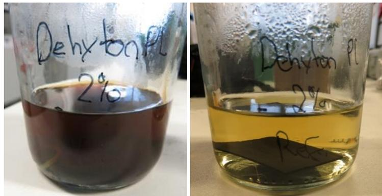
Figure 2. Seals made of FKM (left) and EPDM (right) kept in Dehyton PL at 90°C for 3 days. Image courtesy of SKZ.
