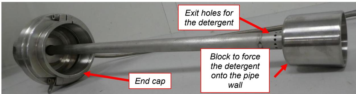
Figure 3. Internal system to spray the detergent solution directly onto the inner side of the pipe wall.
