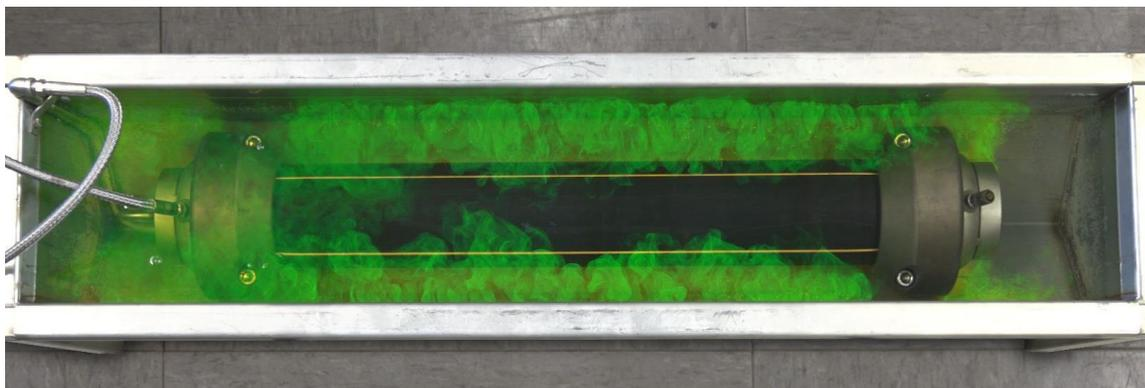
*Figure 8. Checking the flow with a colorant in a smaller tank for the aNPT. A few seconds after this photo was taken, the green colorant was homogeneously distributed.*
