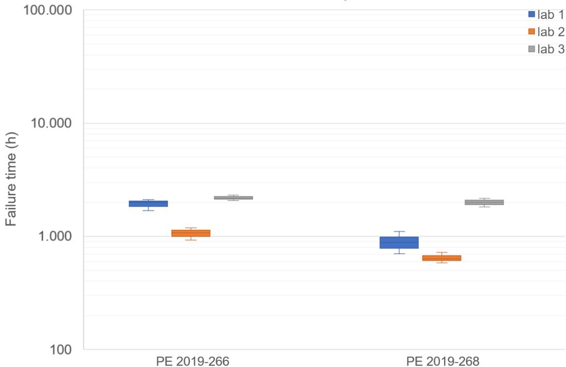
Figure 7. Failure times of two PE pipes tested at three laboratories with 2% Arkopal N100, 4 MPa at 80°C.
