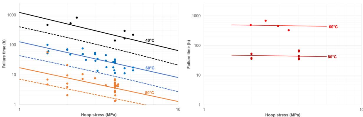
Figure 4. PLT results for first-generation HDPE (left) and second-generation HDPE (right).
