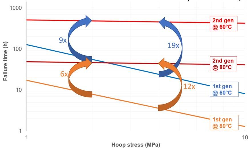
Figure 5. "Generation factor" for two temperatures (60 and 80°C) and two stresses (2 and 4 MPa).
