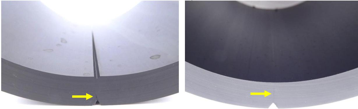
Figure 11. Pipe failure after the aNPT. Left: a non-failed notch has a starting crack (yellow arrow) and an indentation on the inner pipe wall. Right: a non-failed notch has no crack, but a fine line over the ligament is visible (yellow arrow).
