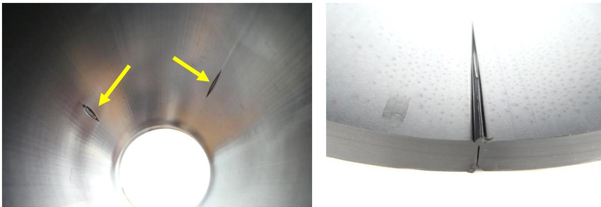
Figure 10. Pipe failure after the aNPT. Left: multiple notches are visible (yellow arrows), although only one failed. Right: the failed notch has a ductile part on the inner pipe wall.
