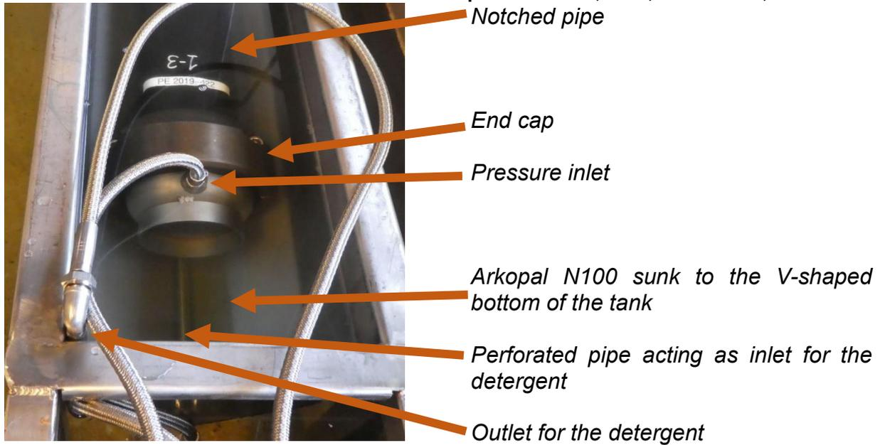
Figure 9. The smaller test setup at Kiwa Technology for the aNPT. In this photo, it is placed outside the water tank and the circulation is stopped, causing segregation of the Arkopal N100 solution.
