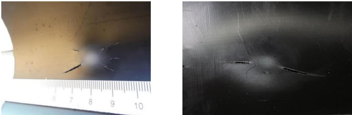
Figure 6. Inner pipe wall under the point load of a failed pipe, tested at lab1 (left) and lab2 (right).
