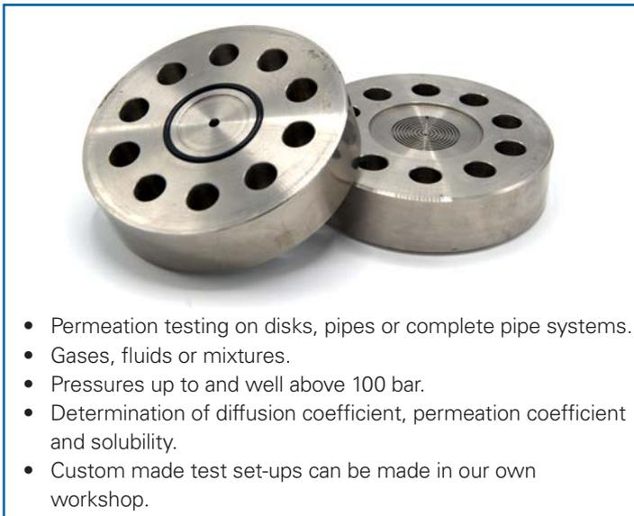
In time test specimen can be taken out of the set-up to perform chemical analyses or mechanical tests in order to identify and quantify any aging effects.
