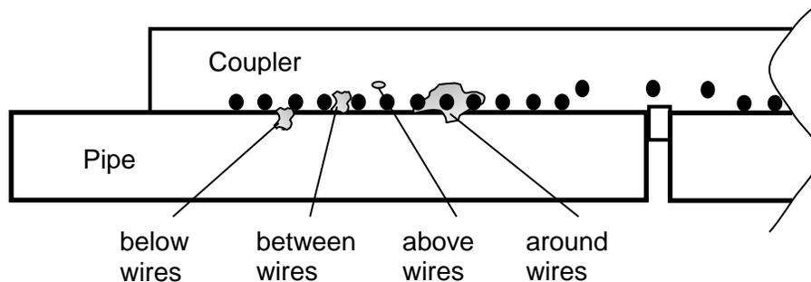
**Figure 2: Possible positions of anomalies in reference to the heating wires**
