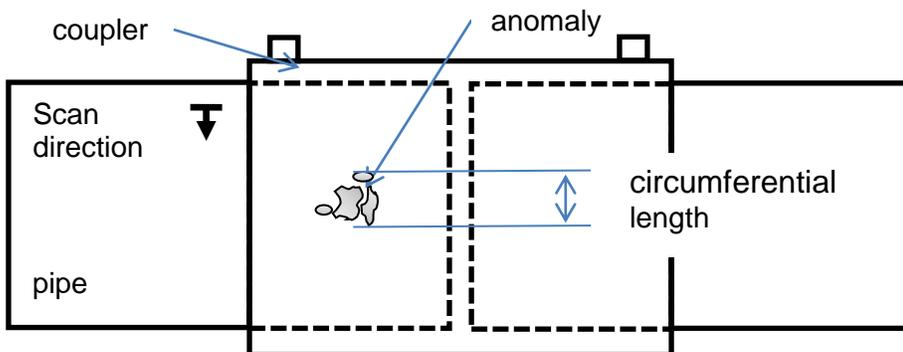
**Figure 4: Measurement of the circumferential length**
