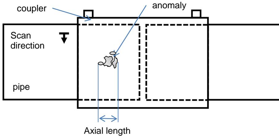
**Figure 3: Axial length of the anomaly**
