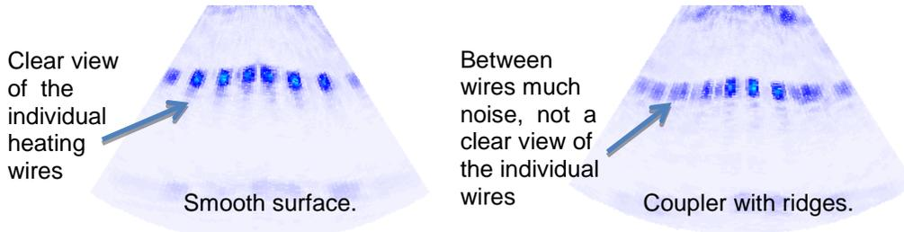
**Figure 5: PAUT image of a coupler with a smooth surface and a coupler with ridges. The ridges of the coupler causes noise in the PAUT image.**
