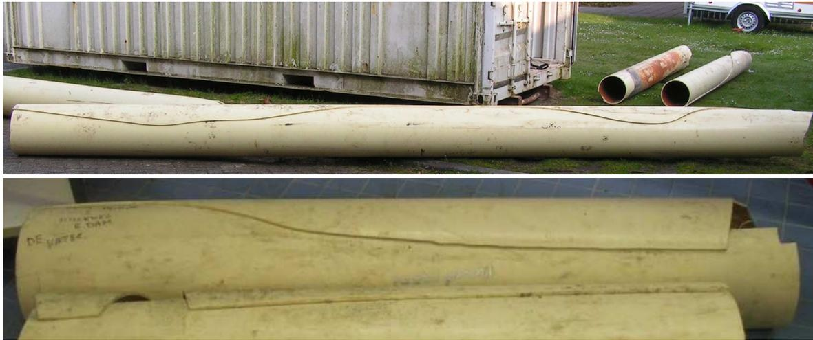
Figure 11. Several uPVC water pipes after RCP in practice. Crack length up to 10 meters.
