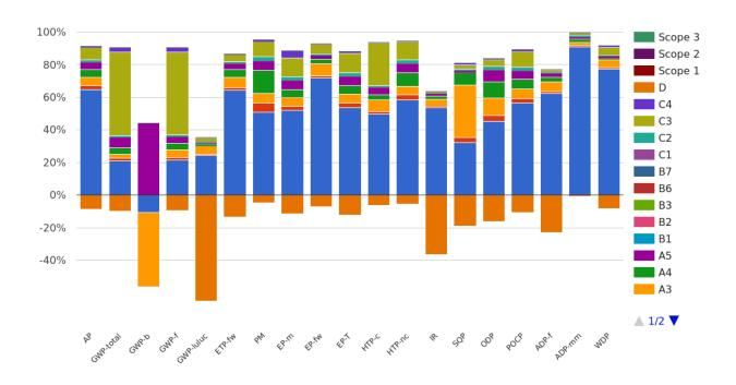
In the case of most of the impact categories, Al is the module that is dominating the impact. GWP total results are to highest extent influenced by module C3 followed by modules Al and A5.
