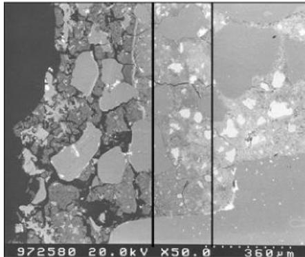
**Fig. 6:** 1st and 2nd damage front, determined on a thin grinding (SEM picture)
