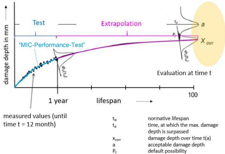
**Fig. 7:** Graphic representation of the damage depths up to 1 year
