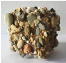
**Fig. 1:** Corrosion examples on concrete when stored in sulfuric acid:
