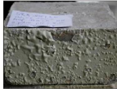
**Fig. 2:** Examples of corrosion after the storage of polymers in sulfuric acid: tensile strength of the material is an essential indicator of the corrosion process, as well as the possible occurrence of brittleness with the peeling off the coating (here pH: 1)
