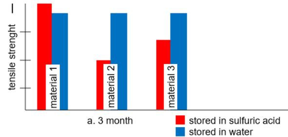
The resistance performance and durability of construction materials against the above-mentioned stress in the area of BSA can be evaluated by a variety of test methods. The materials usually undergo long-term and time-lapse tests in sulfuric acid with different pH values as well as other test scenarios. These tests are partially regulated by normative standards. The evaluation criteria are determined depending on the material and the test procedure used.
