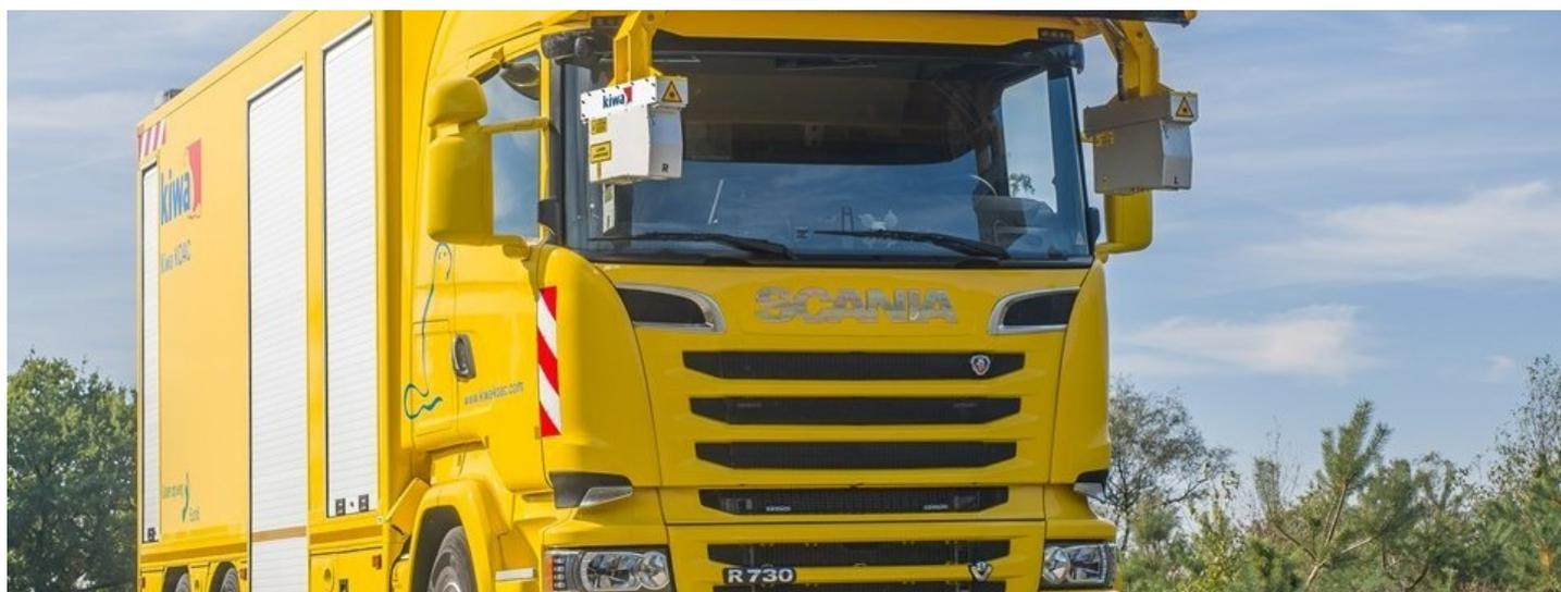
**The SKM grip measurement measures the frictional resistance or force transmission between the measuring tyre and the road surface. The grip varies depending on the condition of the road and the speed of the vehicle.**
