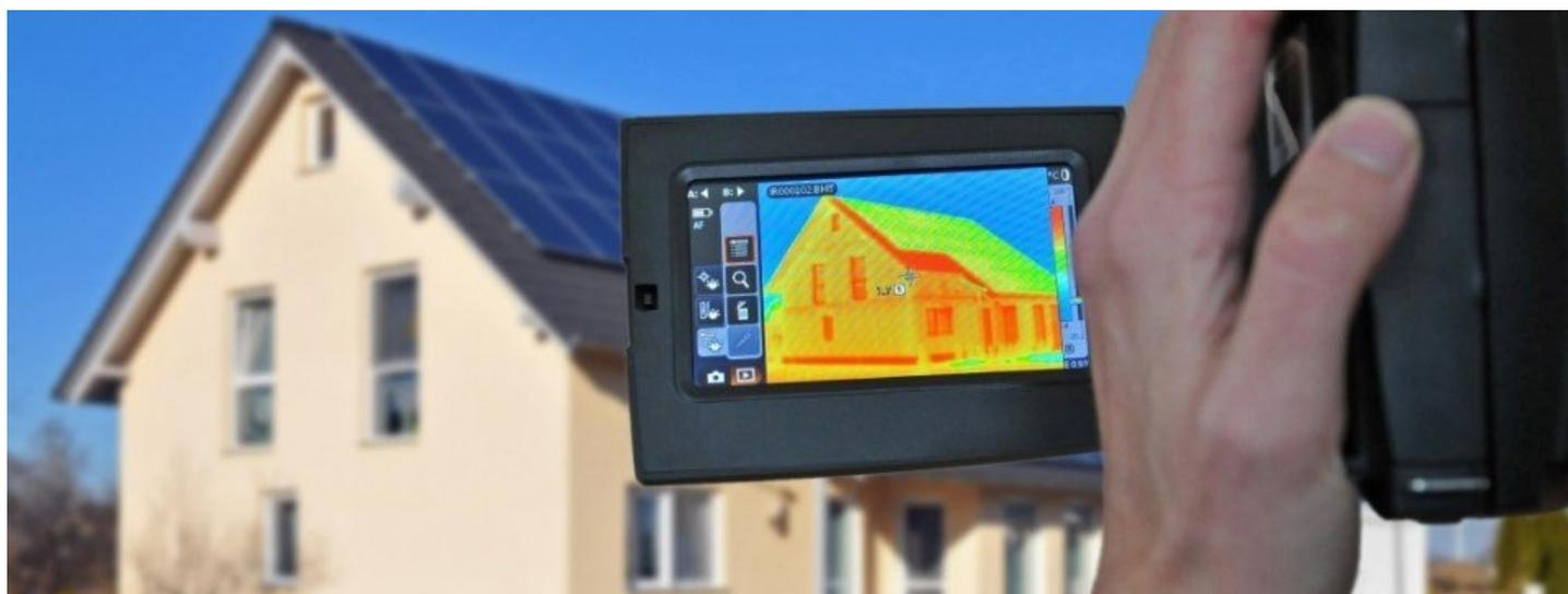
**Heat loss occurs in all buildings. An infrared camera can be used to visualise this heat loss, which is invisible to the eye.**
