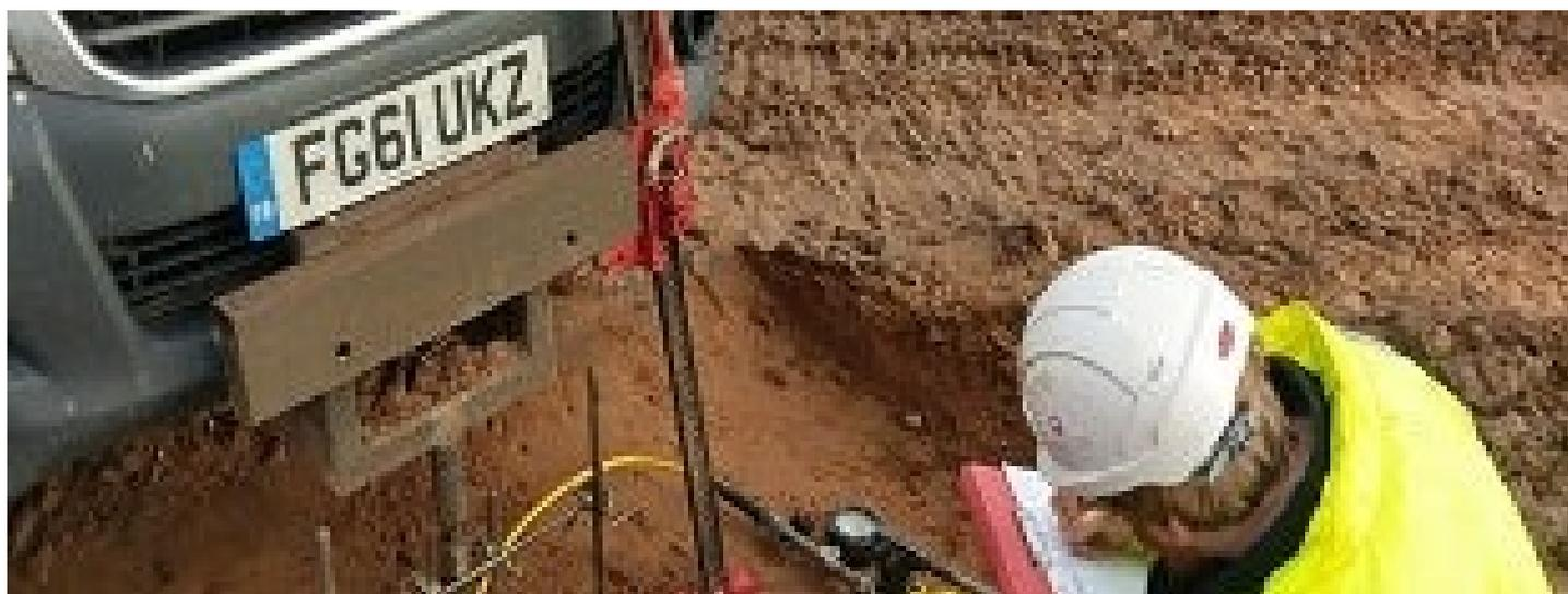
**The Plate Bearing Test is an in situ test used to determine the likely settlement of the ground under a given pressure. Typical applications of the test are for the design of temporary working platforms for crane outriggers, piling rigs etc, determination of the equivalent CBR value when the material is too granular for standard in situ CBRs to be carried out, for instance on subbase materials.**
