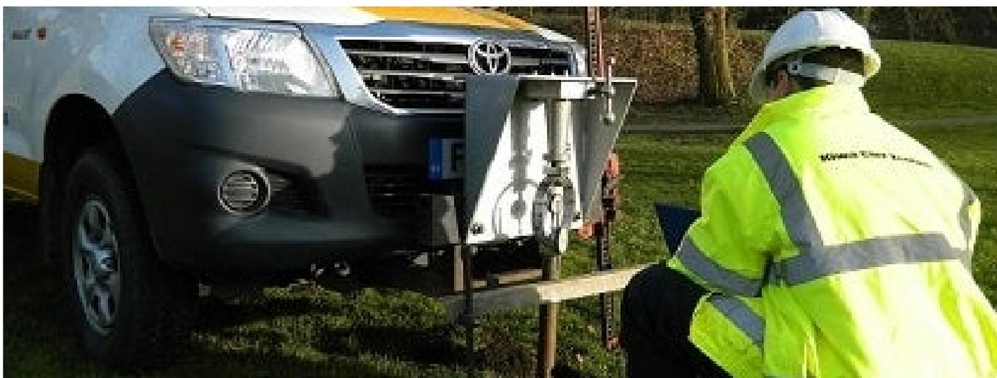
**The in-situ CBR test (California Bearing Ratio) is a simple soil test that compares the bearing capacity of a material with that of a well-graded crushed stone (a high quality crushed stone material should have a CBR of 100%).**
