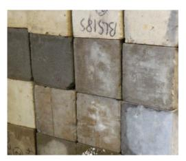
test failures, some deviation from BS:EN12390 has occured in the on-site sampling, compaction and curing procedures. Our trained technicians, who can be mobilised at short notice to visit sites, will carry out the sampling and making of concrete test cubes, which are cured and tested in strict accordance with BS:EN12390 at our UKAS accredited laboratory.
