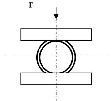
Figure 1 – test set-up for compression
