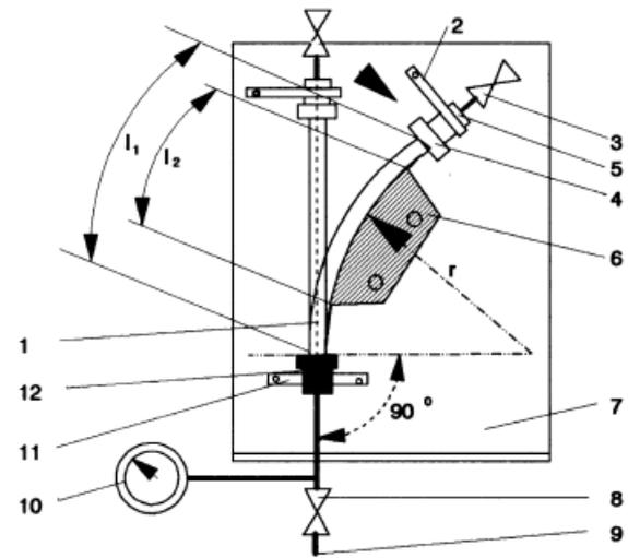
Figure 1 – Bending template
