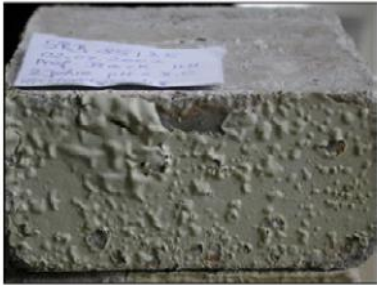
Fig. 2: Examples of corrosion after the storage of polymers in sulfuric acid: tensile strength of the material is an essential indicator of the corrosion process, as well as the possible occurrence of brittleness with the peeling off the coating (here pH: 1)
