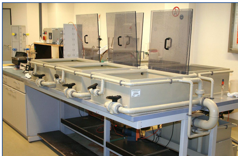
Figure 4: Storage of concrete test specimens for 12 weeks in sulphuric acid, usually with a pH of 3.5
