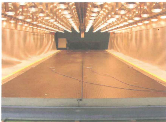
Fig. 2 – Thermal shock test during heating
