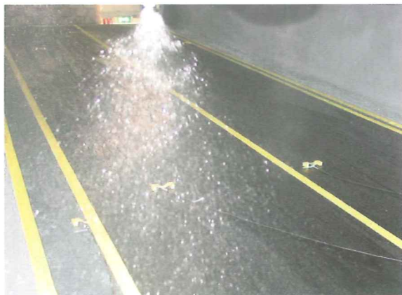
Fig. 3 – Thermal shock test during cooling down
