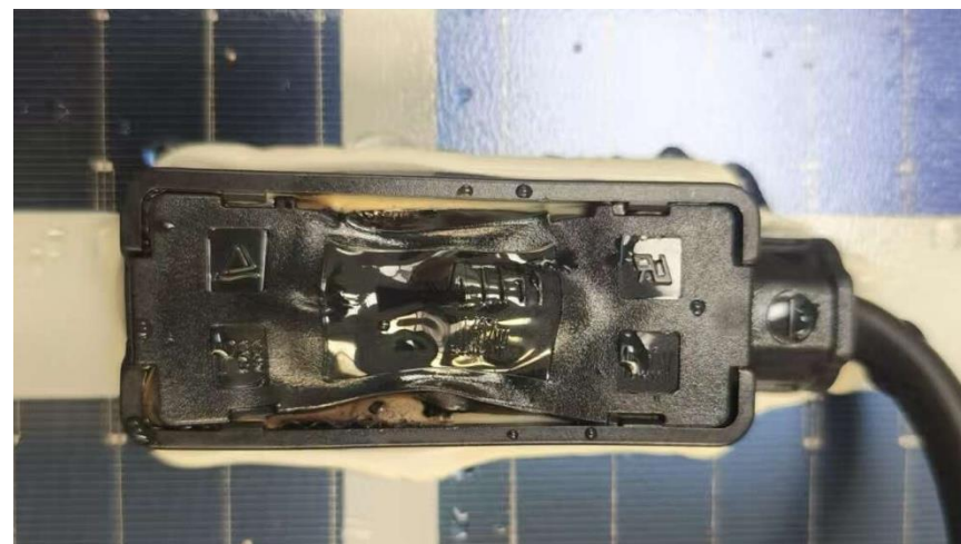
Diode – failed diode after TC200
